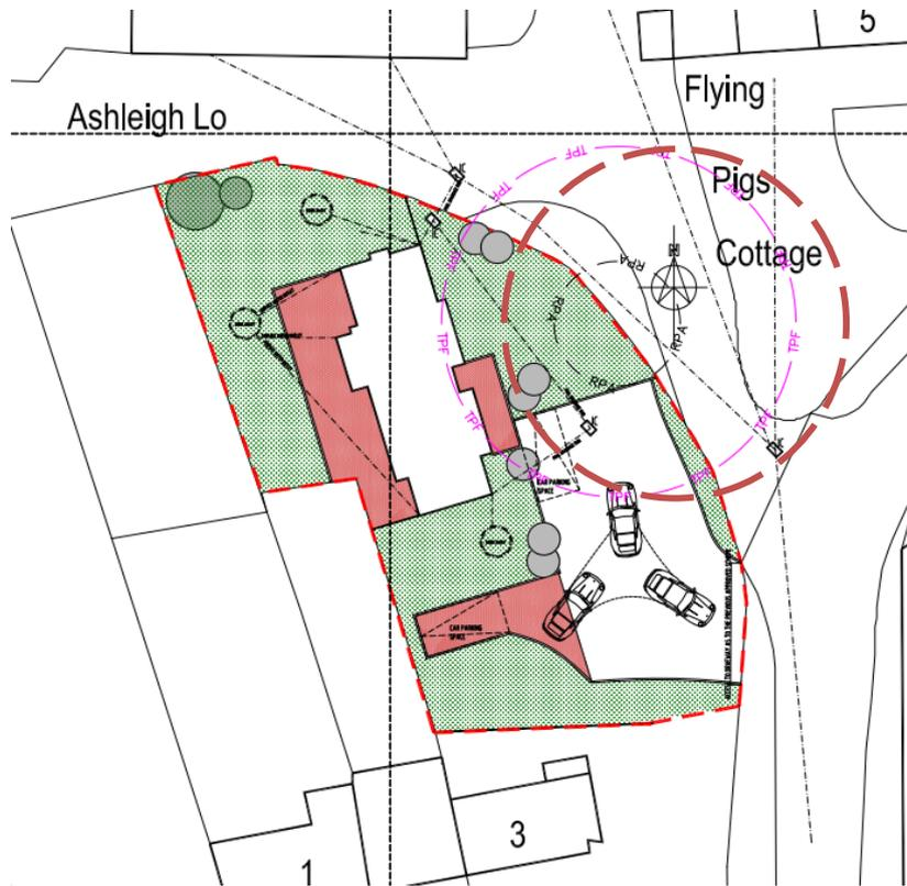
The only aspect of the works that would be within the root protection area is the proposed driveway. This is therefore proposed to be constructed with a cellular design to prevent ground compaction to the surface of the driveway by vehicles, thus protecting tree roots below ground. The cellular design is illustrated at Appendix E. This will be conditioned in the event of an approval.
