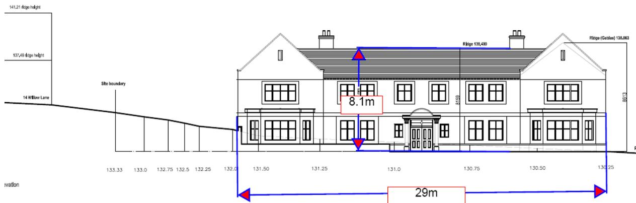
Proposed Front Elevation (showing comparative height to properties on Mill Lane)
