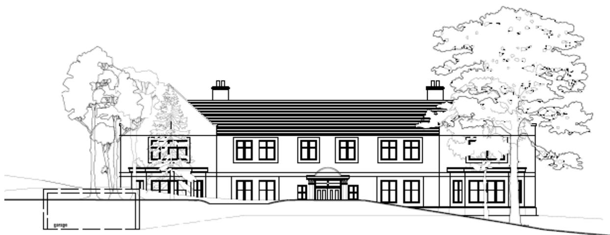
Proposed Front Elevation (in context of ground levels and showing sunken garage)
