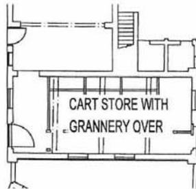
This two storey building has been added to the end of the west barn in the same bricks but uses an improved brick bond style of Flemish garden wall. The gable ends have the same parapet detail as the north barn with stone capping so it is likely to be of a similar date. It has higher eaves than the barns and brick piers on the corners. Access to the first floor is via the external brickwork steps which have a low lean-to adjacent to it presumably for pigs or chickens.
